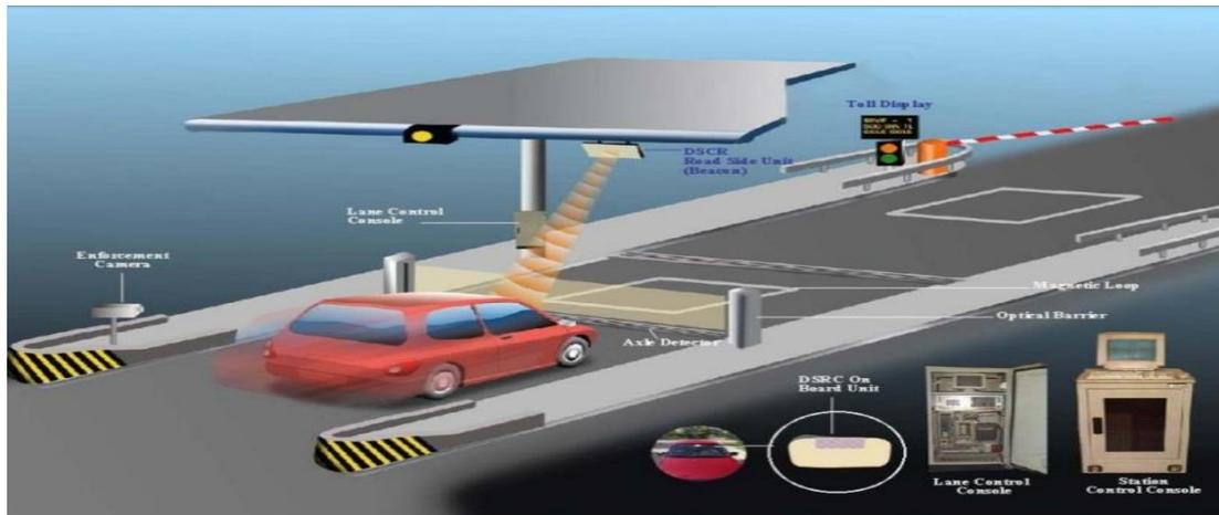
Figure 5: ETC System working principle
