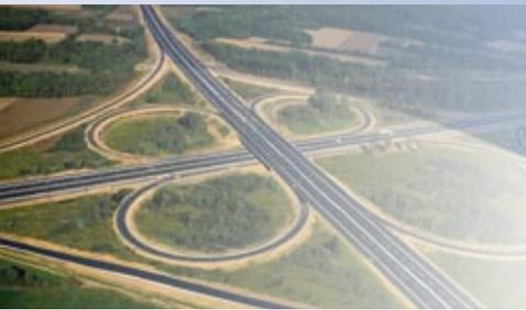
A motorway is an infrastructure specially designed and built for motor traffic and for consistent vehicle classes, according to the highest quality and technological standards, in order to guarantee to all the users the best safety conditions, high levels of service and driving comfort. Actually, motorways are provided with dual carriageways for the two directions of traffic flows, completely separated by a central reserve and with
