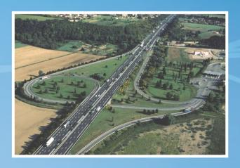
Motorways are characterised by dual carriageways for the two directions of flows (completely separated by a central reserve), the lack of intersections at level, proper lanes for on/off merging and the presence of grade-separated interchanges
