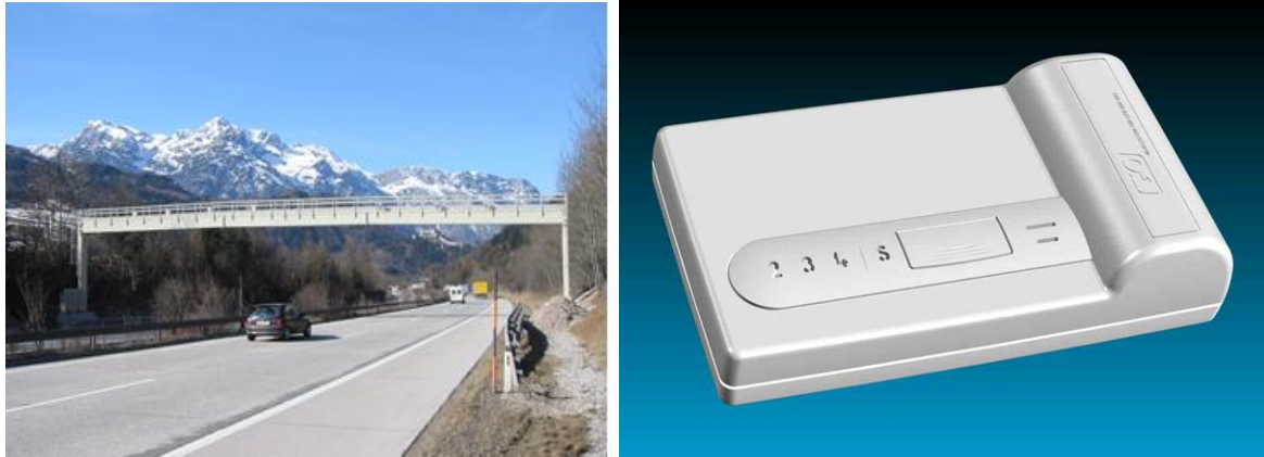
Figure 18: An Austrian tolling gantry and the GO-Box (Austrian OBU)
